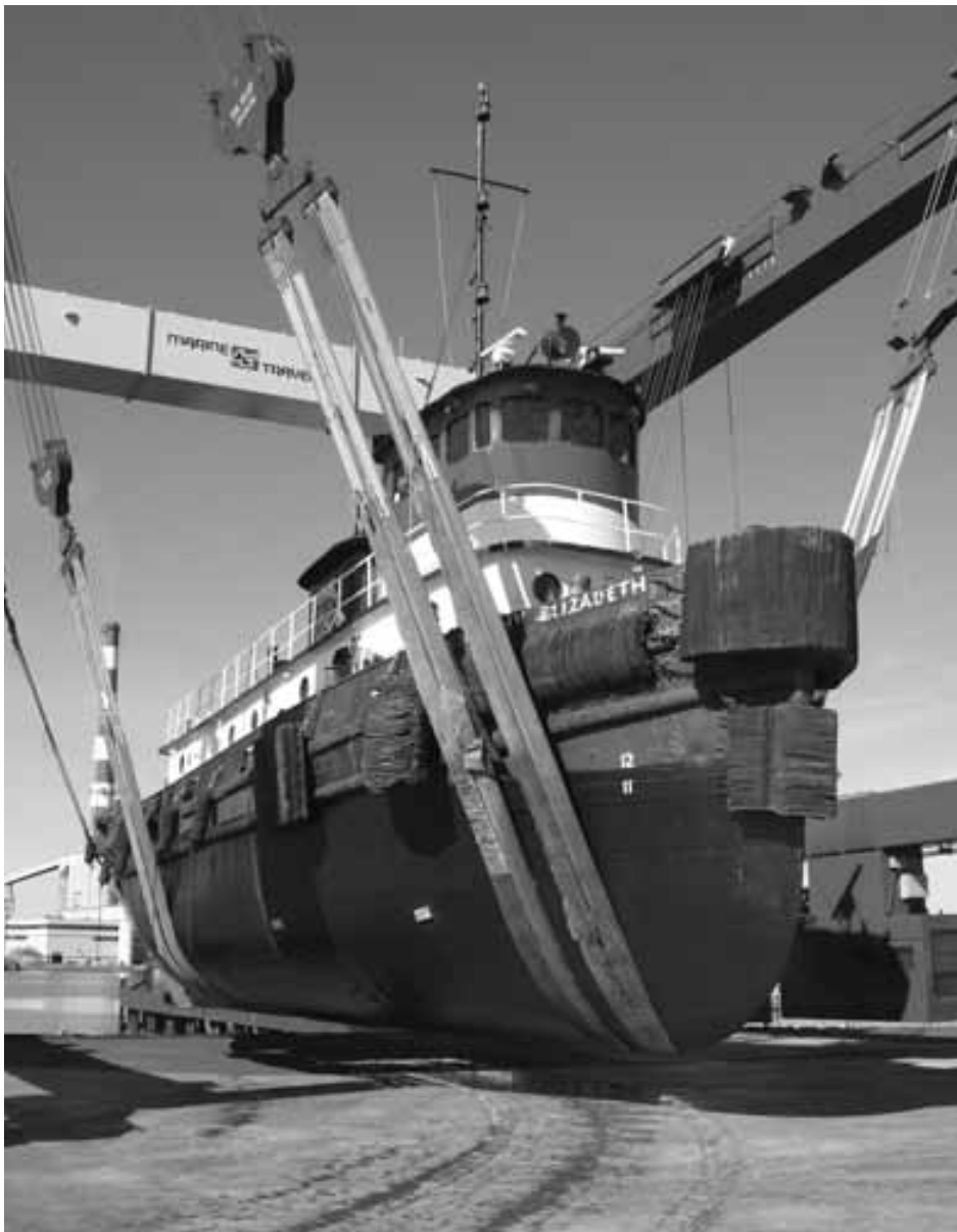
A six-hour ride from the "port city" of New York, the 600-ton Travel Lift at the Derektor yard in Bridgeport, Conn. eases the freshly scraped and repaired Dorothy Elizabeth back to the water. (Photo: Don Sutherland.)
