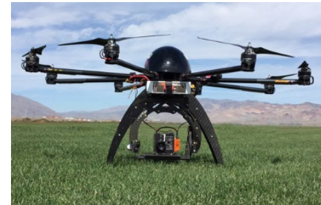
UAS equipped with Hyperspectral Imager (Source: Headwall Inc)
